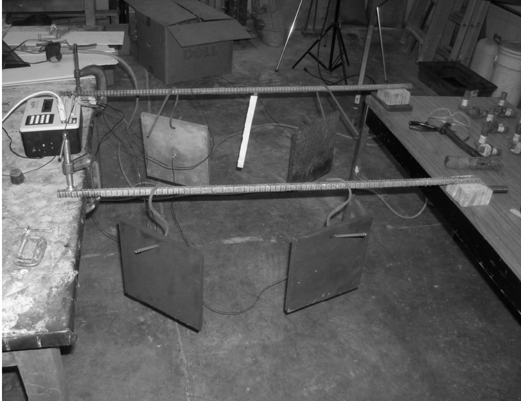
Figure 3.15 Photograph of Test Plates Hanging After Being Heated in an Oven
